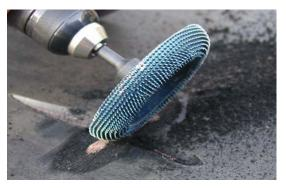
The surface should then be cleaned off with a suitable solvent e.g Trichloroethylene or Methyl Ketone (MEK). The bonding layer must be removed using a suitable de-greasing solvent.
