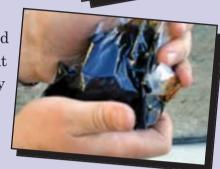
Cut open any corner with a knife or pair of scissors. Squeeze out the resin onto the worn area.
