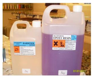
Mixing ratio is 2:1 by volume, mixing time is 3-4 mins until uniform colour and streak-free
